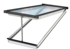
Motorized smoke venting skylight module. Actuator chain stroke up to 700 mm, which opens in less than 60 seconds. Only open system actuator available.
