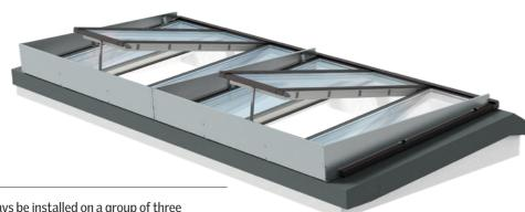
Wind deflector KCD 0080 must always be installed on a group of three skylight modules with identical width, where the middle module is the smoke ventilator and the two modules at the sides are fixed modules. This deflector is manufactured to fit the size of the three modules it is
